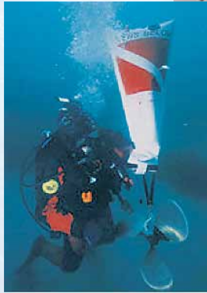
Using a Quad Bag to raise a propeller.
