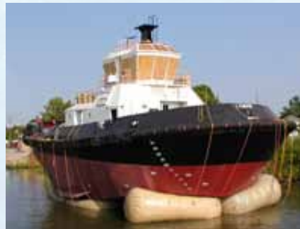
Salvage pontoons used to reduce draft of tugboat during launch.
