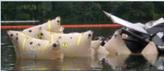
Enclosed Flotation Bags used to raise a downed helicopter by Italia Fire Brigade.
