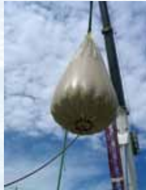
Used as a water Test Weight Bag for cranes, life boats, davits, etc.
