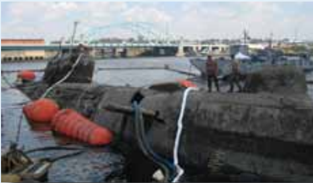
US Navy using Salvage Pontoons to raise 9,000 ton Russian submarine
